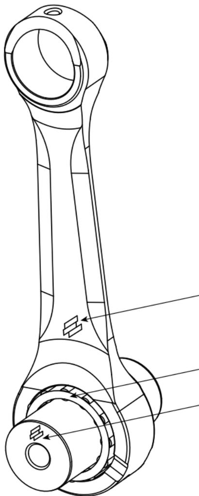
ASSEMBLE IT WITH THE MARKING ON THE SAME SIDE.
