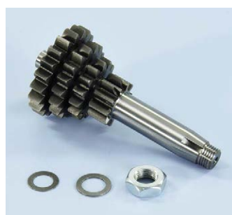
202.1417 Vespa 50/125 ET3 Z=10-14-17-20 Primary ratio-Primario
